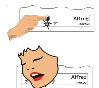
Speak your message as close as possible into the microphone. The record lenght is about 60 seconds. As the red LED will start flashing, you will have 5 secondes of recording time left.
